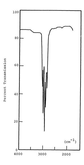
Fig. 1. Infrared spectrum of the product obtained in the exchange reaction of ethylbenzene with  $\rm D_2O$  over the Sn-P(10/1) catalyst in the C-H and C-D stretching vibration regions.
